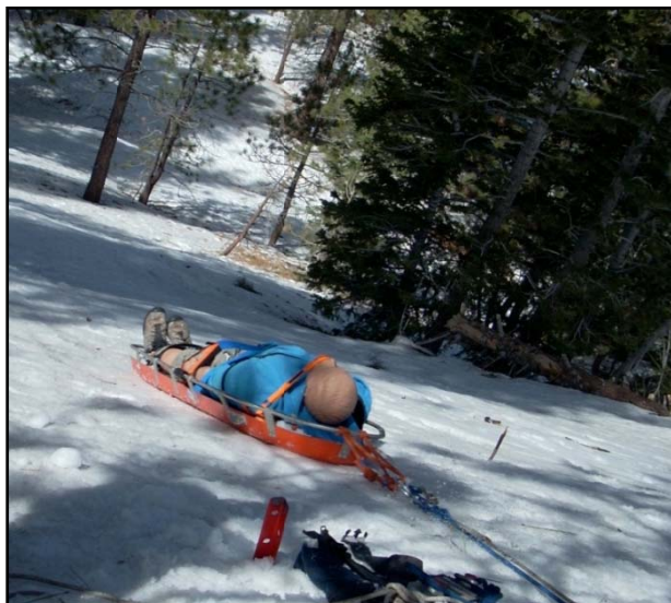
Figure 1. Drop testing with a loaded litter on a snow slope.
