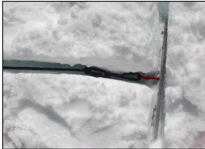
Figure 3. Top view of a horizontal picket placement
