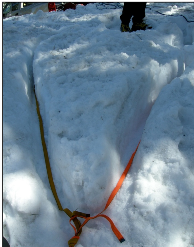
Figure 5. Bollard prior to drop testing. Note the lack of padding between the webbing and the snow.
