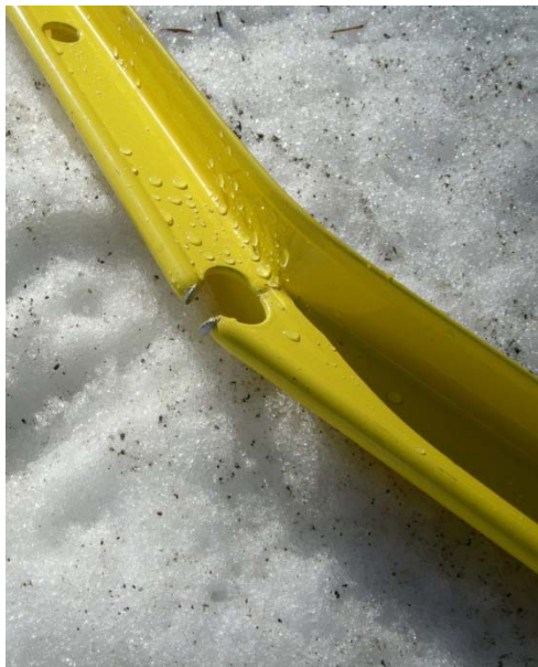
Figure 9. 3-foot horizontal picket after testing. The carabiner hole failed at a peak impact load of 960 lb.
