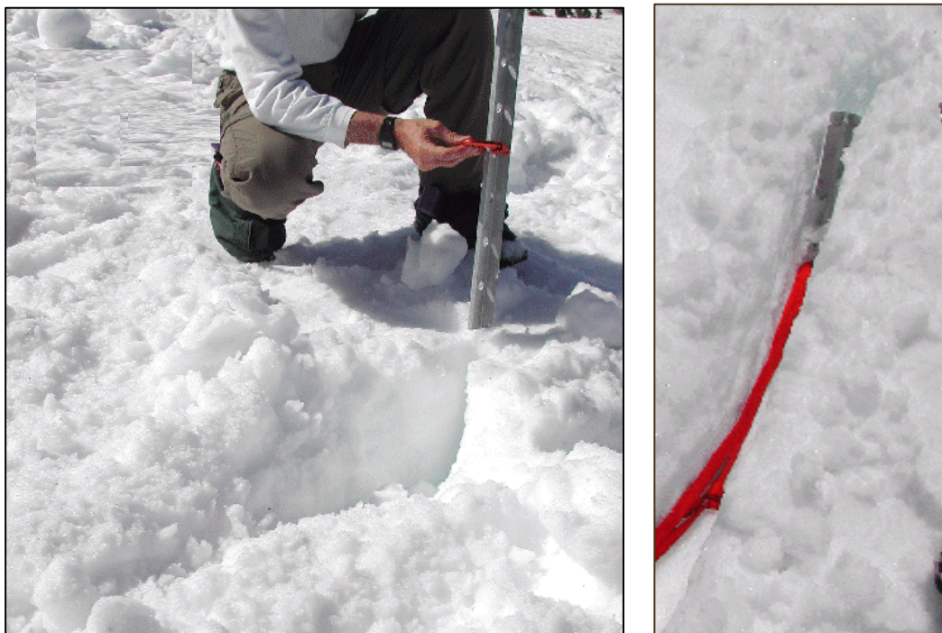
Figure 4. View of Sierra Picket prior to and after placement.
