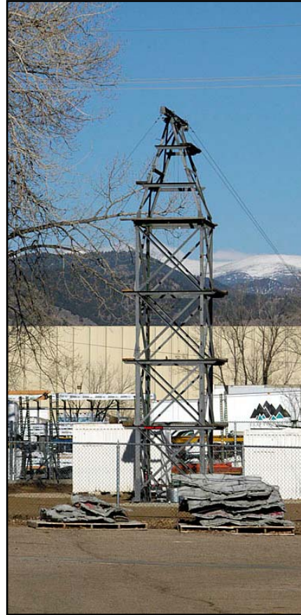
Figure 1: The RMRG test facility includes a 35' (10.7m) tall test tower, with 1000 lb (4.45N) of steel weights and a built-in hoist.
