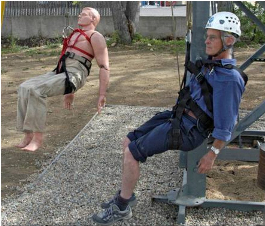
Figure 2: The Rescue Randy mannequins were typically fitted with a chest harness to better emulate a rescuer's body position.
