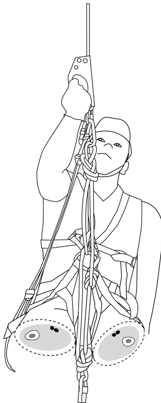
Figure 2. Leg vessels in relation to harness straps.
